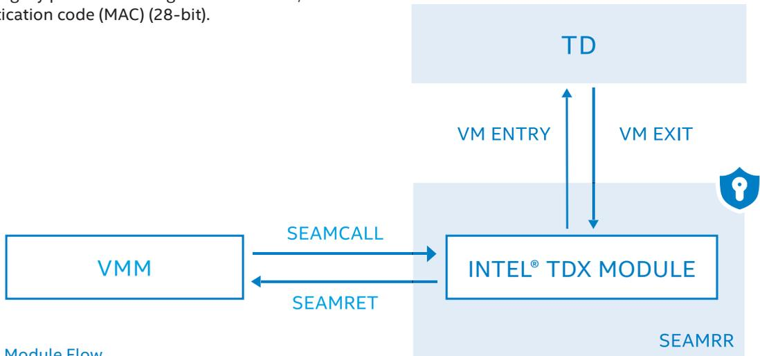
Figure 5.2. SEAM Module Flow
