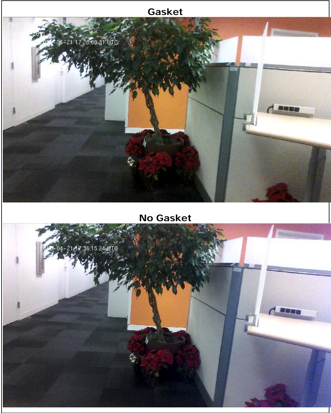
Figure 7-6. Example of Light Leakage Effects
