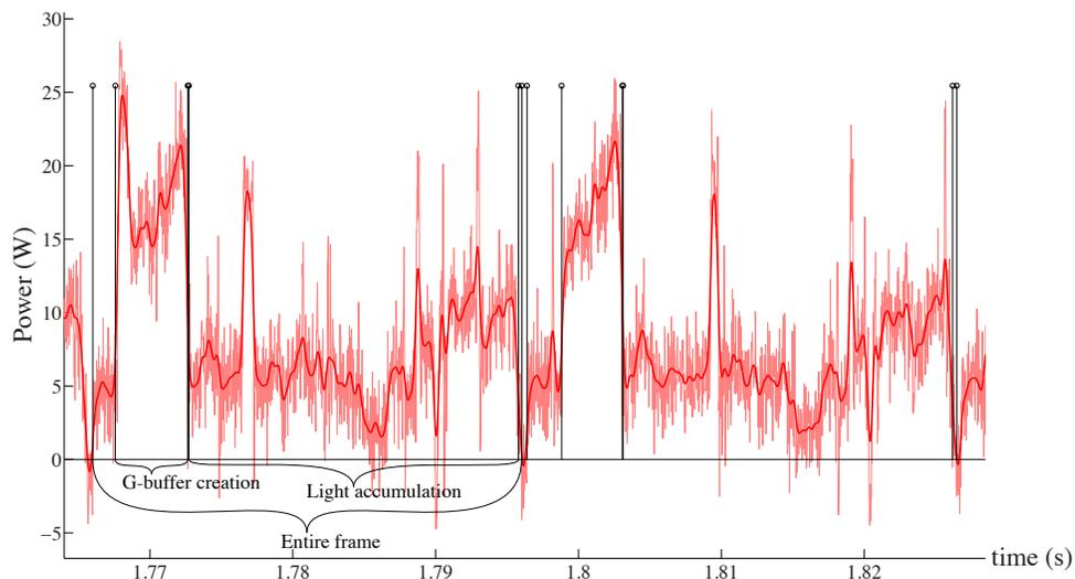
**Figure 1.** Measured power for deferred shading on an Ivy Bridge processor. The entire frame on the left uses 135 nJ/pixel. The G-buffer creation pass uses 47 nJ/pixel and the light-accumulation pass uses 84 nJ/pixel. Note that the removal of the CPU power pushes the curves below zero at times. This is because the idle power that is removed is an average over several complete frames, which reduces noise in the graphs (but still gives a correct average energy per pixel).
