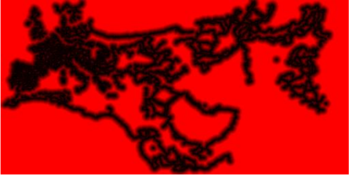
Figure 12. Final Distance Field Texture. Each pixel holds the distance to the nearest border.
