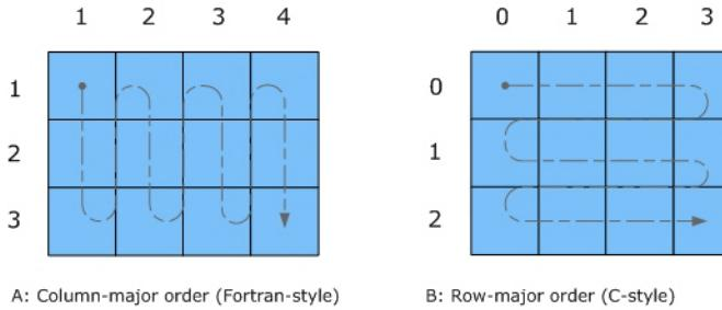
For example, if a two-dimensional matrix A of size  $m \times n$  is stored densely in a one-dimensional array B, you can access a matrix element like this:
