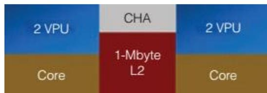
Figure 2. Intel® Xeon Phi™ processor illustration of a tile from Figure 1 that contains two cores (CHA = Caching/Home Agent, VPU = Vector Processing Unit) [1].
