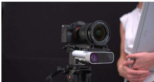
Figure 3. All the user needs are a depth camera, an optional digital camera, and a laptop or tablet (Azure Kinect DK pre-production device shown)
