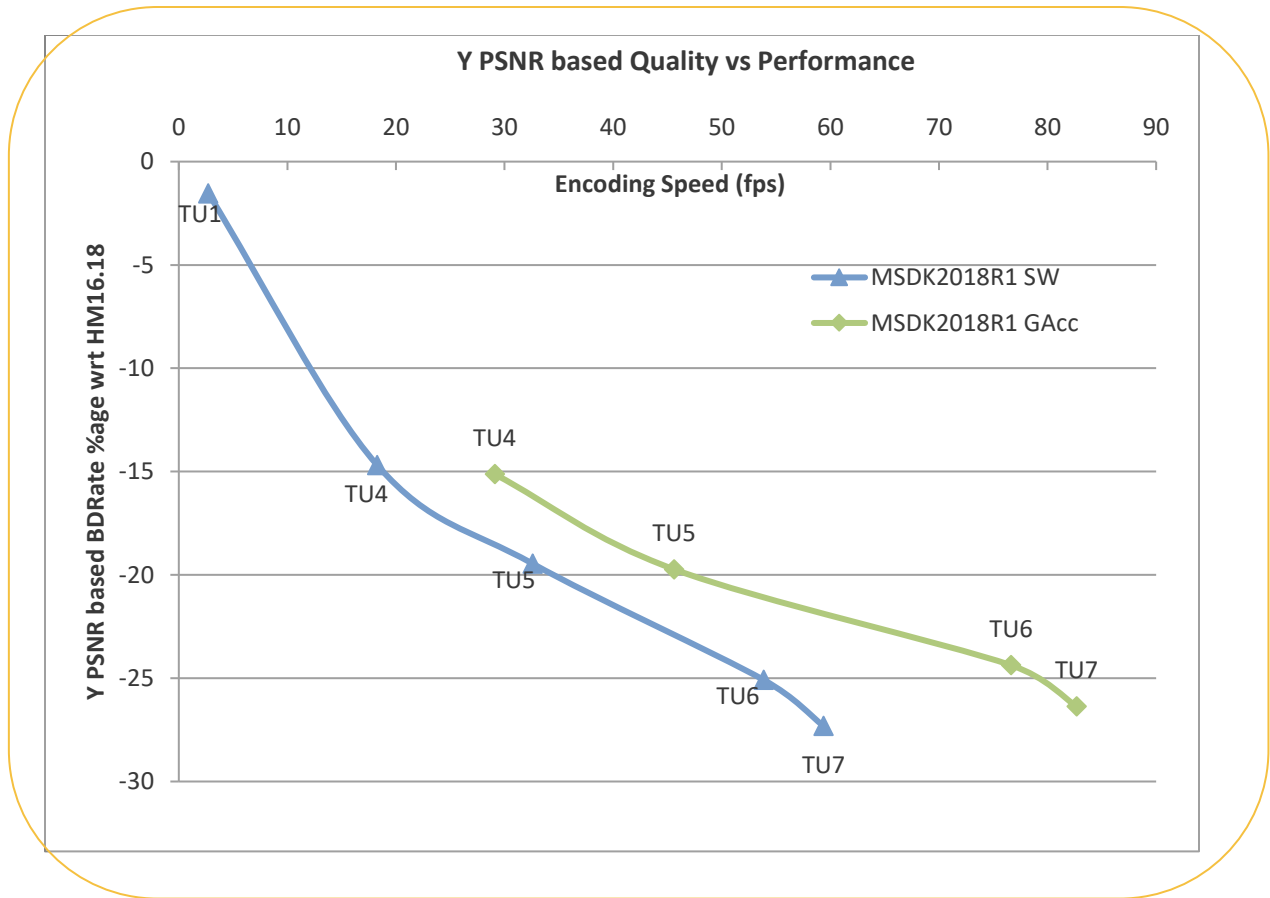
Figure 9A Quality (Y PSNR based BD rate wrt HM16.18) vs Encoding Speed Tradeoff in encoding of HD1080p content by MSS HEVC Software, and MSS HEVC GAcc Encoders in different TU modes, on test system configuration 2 (cfg2)
