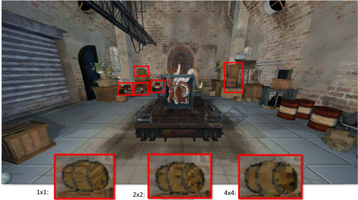
Figure 3. We modified the multithreading sample in the Microsoft DirectX* 12 SDK samples to leverage VRS on select geometry distant from the camera. At a distance, it is difficult to discern the reduced shading rate of objects. By taking advantage of this we can improve the performance of our application without any perceivable loss in quality.
