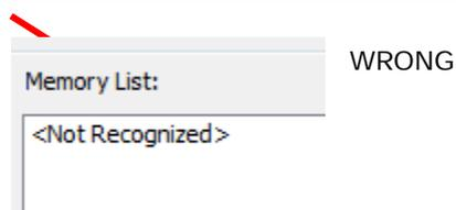
**NOTE:** If you see this, this is WRONG. Be sure to check that the DediProg is connected to the computer and that your DediProg driver is installed. The driver is bundled with the DediProg software installer downloaded from the DediProg website in the WinUSB driver folder.
