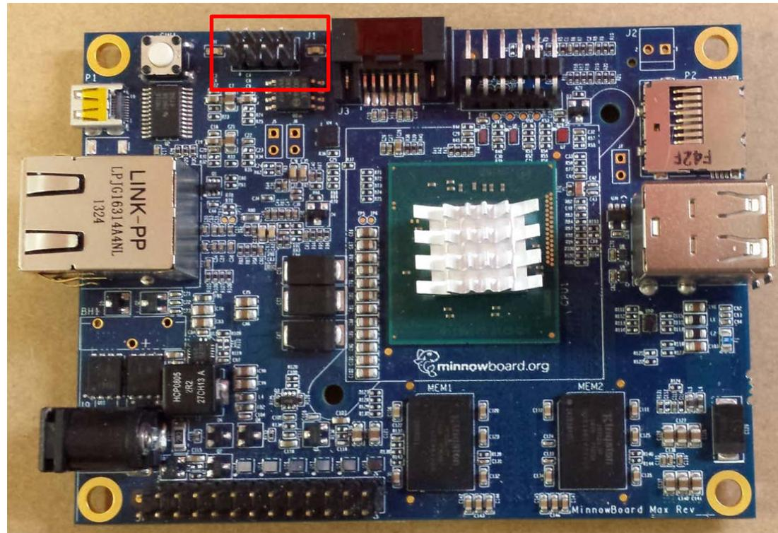
3. **Connect the DediProg cable to the 2x4 PROG header** so that the red wire of the cable is on the pin 1 side of the header that is furthest from the power switch. Pin 1 is next to the SATA connector
