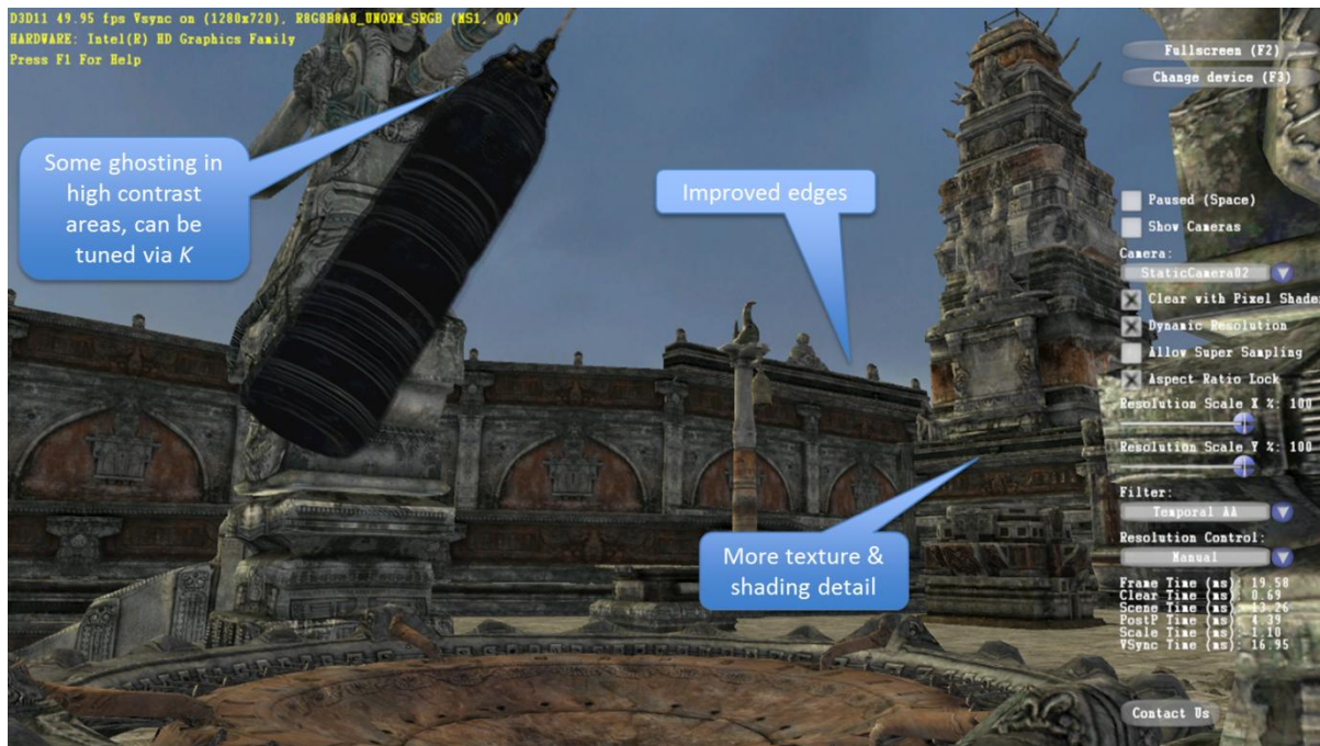
Figure 8: Temporal Anti-Aliasing with velocity scaling and moving objects
