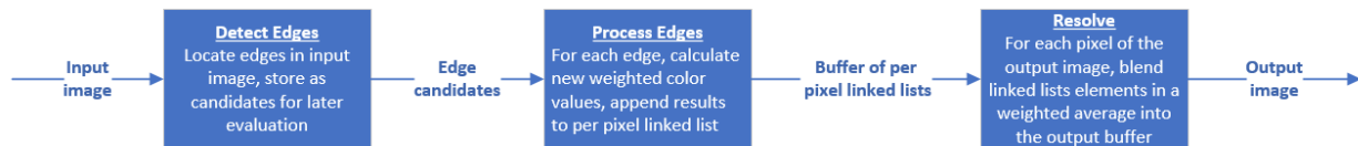
Figure 3. An overview of the three primary stages of the CMAA 2.0 algorithm. Each stage is an independent compute shader and takes input from the previous stages to compute the final render target. Details of each stage are described below.
