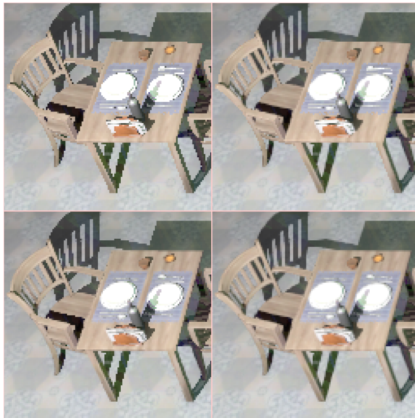
Figure 19. Top left: no AA; Top right: CMAA2 alone; Bottom left: 4xMSAA alone; Bottom right: 4xMSAA+CMAA2. This scene uses exaggerated shadows to demonstrate shader aliasing and is not used for numerical analysis.
