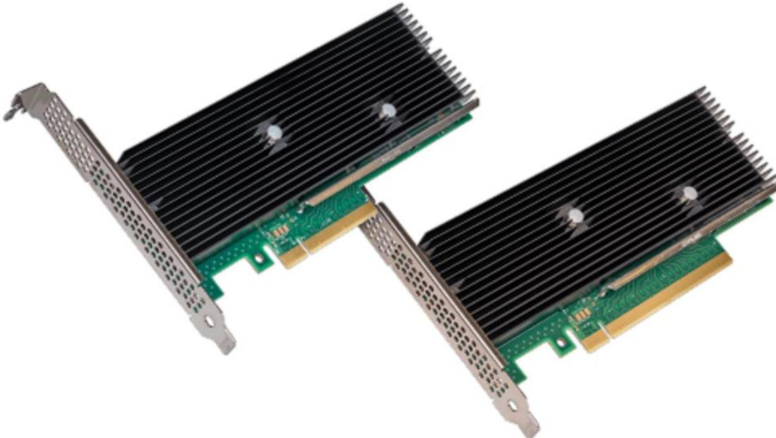
After the card is installed, you need to go to the BIOS settings and set the **PCIe link speed** to **Gen4 and X16** for highest possible performance.
