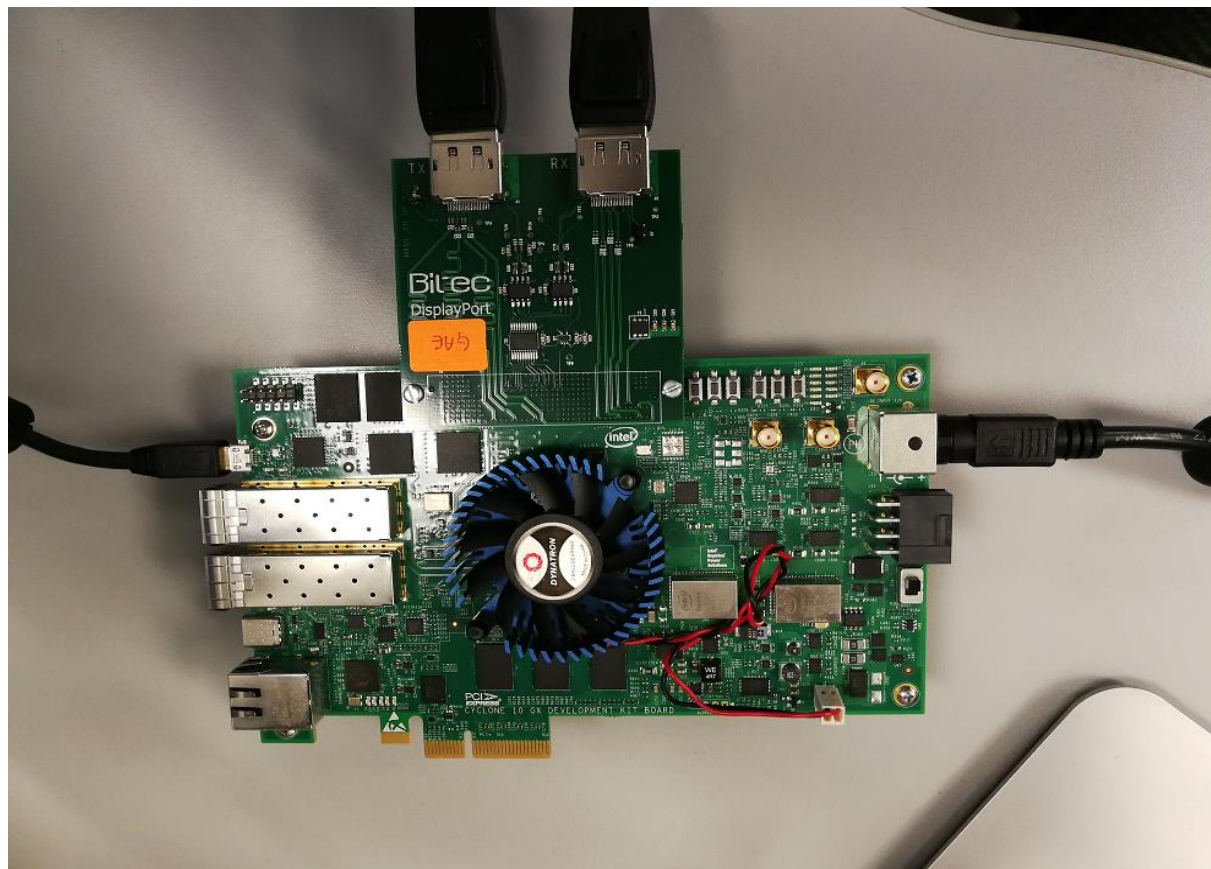
Figure 3. Cyclone 10 GX FPGA Development Kit Hardware Setup
