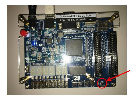
The Max10 has its reset switch on the back of the board as referenced in the documentation. The Cyclone DE0-CV instead has a pushbutton on the front of the board. Its default state is active-low and will only reset when pushed.
