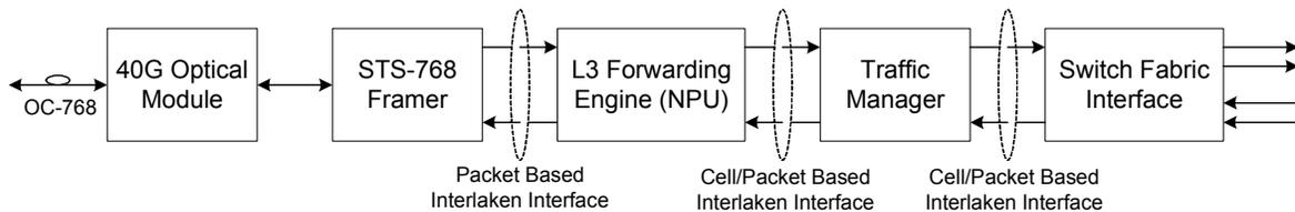
Figure 1. Single Port OC-768 Packet over SONET Line Card
