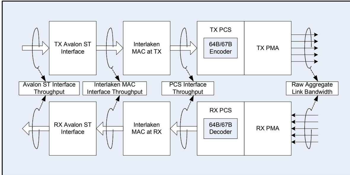
Figure 3. Interlaken Block Diagram and Interface Bandwidth Nodes
