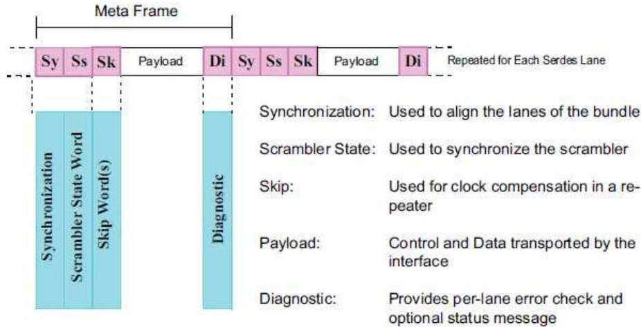
Figure 4. Interlaken Meta Frame Structure from Interlaken Protocol Definition Specification V1.2
