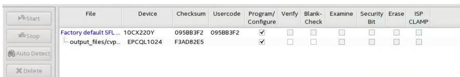
5. After the `.periph.jic` is programmed, the FPGA must be powered cycle to allow the new peripheral image to load from the on-board flash into the FPGA. To force the host PC to re-enumerate the link with the new image, power cycle the DUT PC and the Intel Cyclone 10 GX Development Kit.
