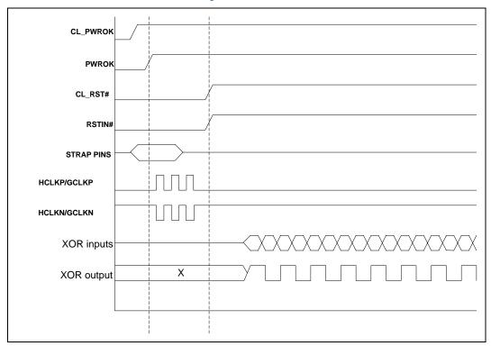
Figure 12-1 shows the wave forms to be able to boot the part into XOR mode. The straps that need to be controlled during this boot process are BSEL[2:0], SDVO\_CTRLDATA, EXP\_EM, EXP\_SLR, and XORTEST.
