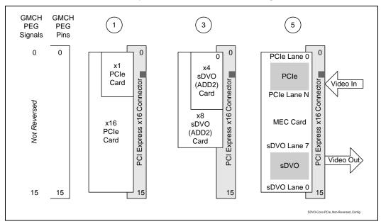
Figure 9-3. Concurrent sDVO / PCI Express\* Reversed Configurations
