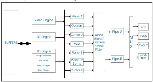
The Mobile Intel GMA X3100 contains a variety of planes, such as display, overlay, cursor and VGA. A plane consists of a rectangular shaped image that has characteristics such as source, size, position, method, and format. These planes get attached to source surfaces, which are rectangular memory surfaces with a similar set of characteristics. They are also associated with a particular destination pipe.
