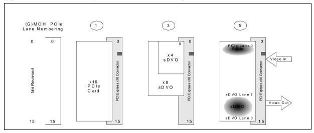
Figure 12. SDVO/PCI Express\* Reversed Configurations
