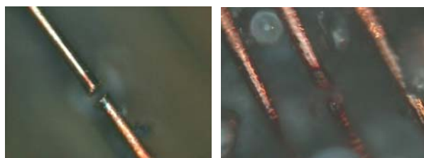
Figure 24: Mold compound removed only at upper right side
