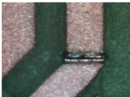
Figure 26: Trace width is approximately 28-microns wide
