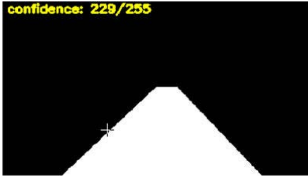
Figure 9: Starting with the clipped probability map (one), the image is first blurred (two), and the edges are fit to straight lines (three). Combining these lines with the effective horizon, a model for the road is constructed (four). A confidence score is assigned based on the number of pixels correctly classified by the implied road structure (four).
