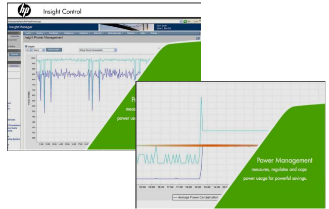
Fig.: HP Insight Control Power Management functionality for Dynamic Power Capping.
