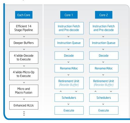
Figure 2. With the Intel Wide Dynamic Execution of the Intel Core microarchitecture, every execution core in a multi-core processor is wider. This allows each core to fetch, dispatch, execute, and return up to four full instructions simultaneously. A single multi-core processor with four cores could fetch, dispatch, execute, and return up to 16 instructions simultaneously.
