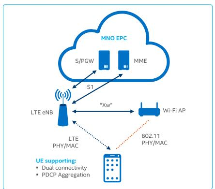
FIGURE 5. LWA CONFIGURATION DEPICTING THE INTERFACES BETWEEN ENB, WI-FI AP, AND UE WITH THE CORE NW FOR A NON-COLLOCATED SCENARIO
