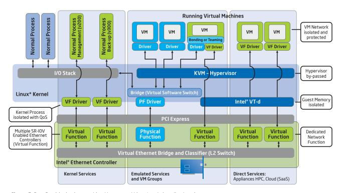
Figure 5. Port Partitioning in a combined bare-metal Linux\* and virtualized environment
