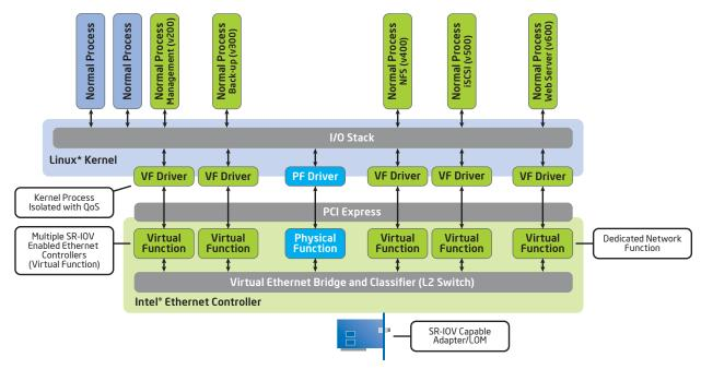
Figure 4. Port Partitioning implemented in a bare-metal Linux\* environment
