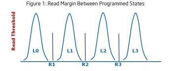
With more P/E cycles, read margin shrinks, resulting in both data retention problems and higher read errors beyond the limit specified by JESD218. This is caused by:
