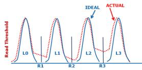
An SSD targeted for client applications may try to overcome these issues using an on-board Error Correction Code (ECC) engine. However, once beyond a certain level of P/E cycles, these SSDs can fail to recover data near the end of life of the SSD. HET uses "beyond ECC" error recovery steps to cross this hurdle of ECC limitation and extend the MLC NAND capability to a higher P/E cycle count.
