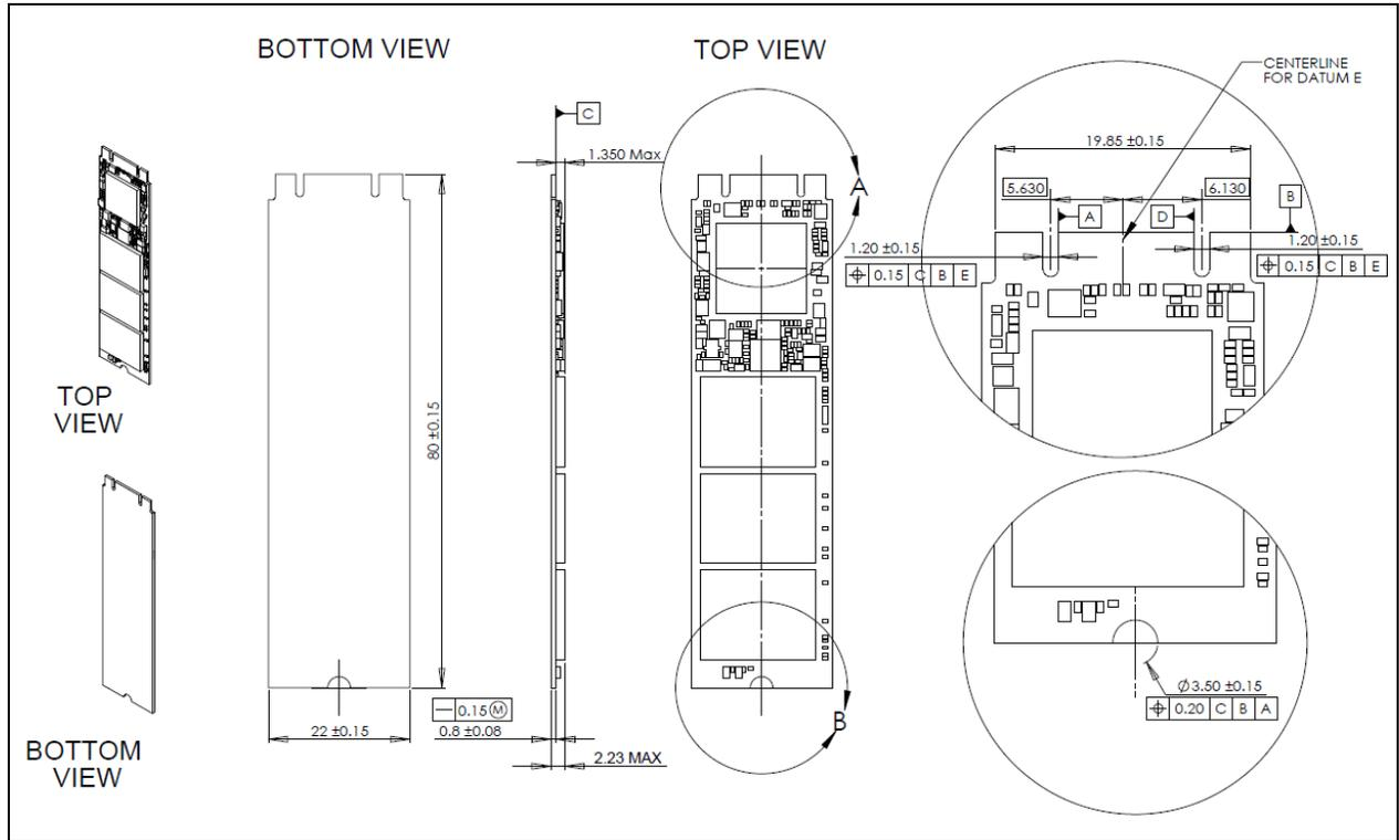
Figure 2: Dimensions for 80 mm double-sided M.2 Form Factor Drives (2280-D2-B-M) 120GB, 240GB, 360GB
