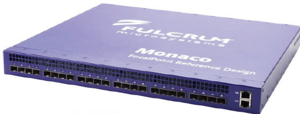
The FM4224 top-of-rack switch reference platform with 24 SFP+ ports.
