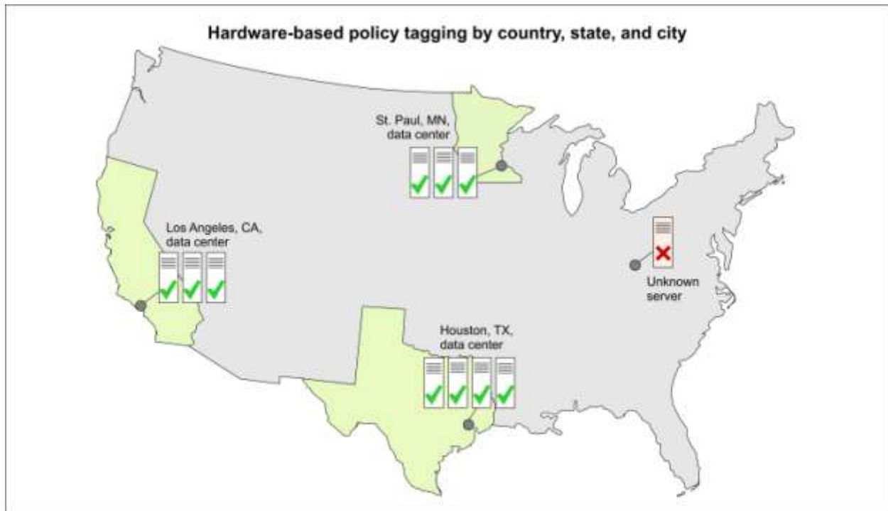
Figure 9. Hardware-based policy tagging. You can tag hosts by country, state, city, region, or special group. Upon boot, hosts not in approved locations or groups can be identified as unknown or not trusted.
