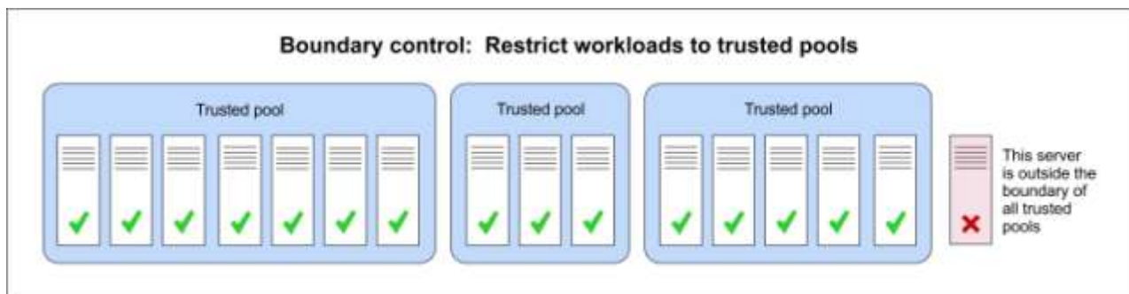
Figure 4. Boundary control. VMware vCenter* allows you to cluster servers, and HyTrust CloudControl (HTCC)* allows you to establish the trusted status of those servers. Combined with the root of trust established by Intel® Trusted Execution Technology (Intel® TXT), these technologies allow you to establish trusted pools of servers. You can then use those trusted pools to help make sure that workloads do not run on machines outside the boundaries of those trusted pools.
