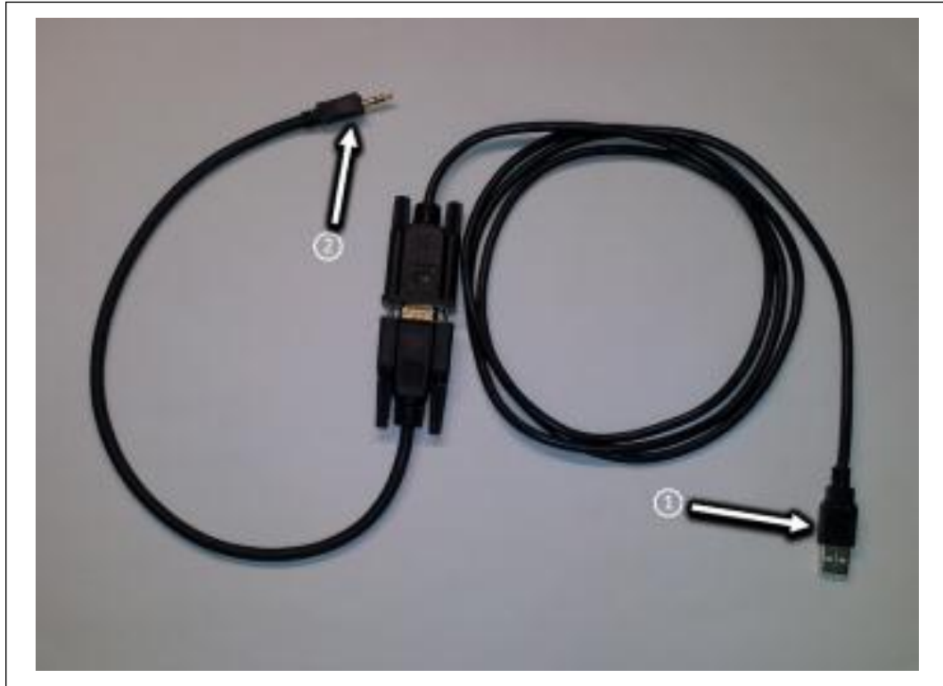
Figure 3. RS-232 Cable for Serial Communication Transmission
