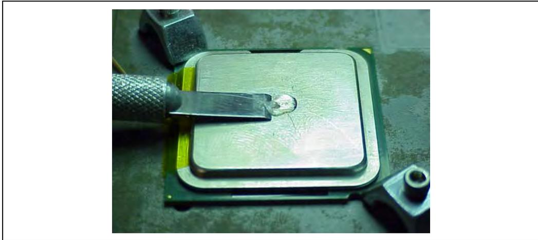
33. Using a blade, carefully shave any adhesive that is above the IHS surface (Figure 57). The preferred method is to shave from the edge to the center of the IHS.
