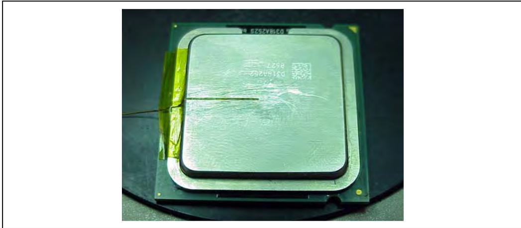
29. Using a blade carefully shave the excess solder above the IHS surface. Only shave in one direction until solder is flush with the groove surface (Figure 54).
