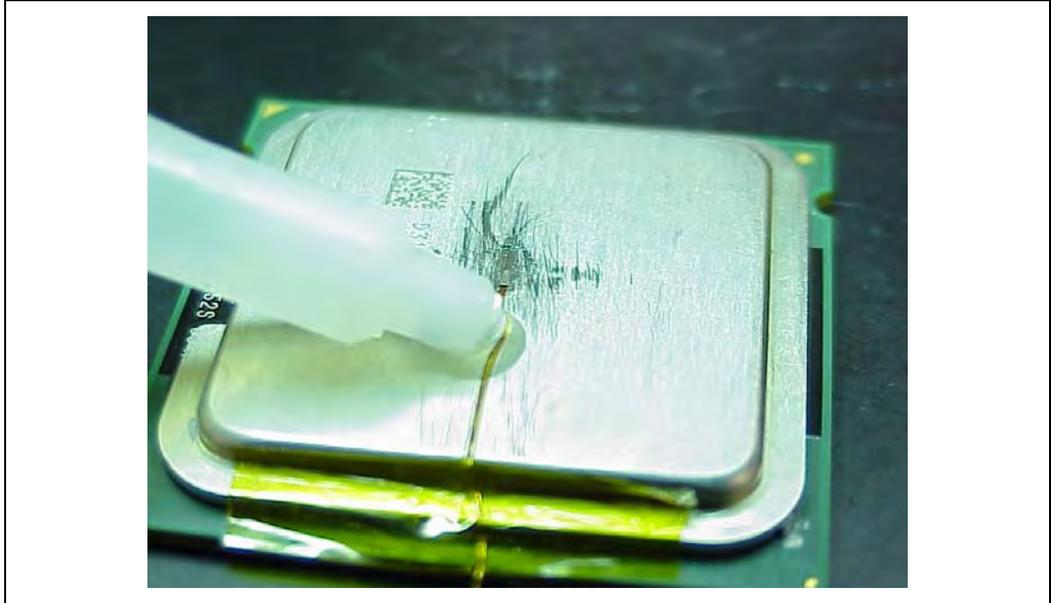
32. To speed up the curing process apply Loctite\* Accelerator on top of the Adhesive and let it set for a couple of minutes (Figure 56).
