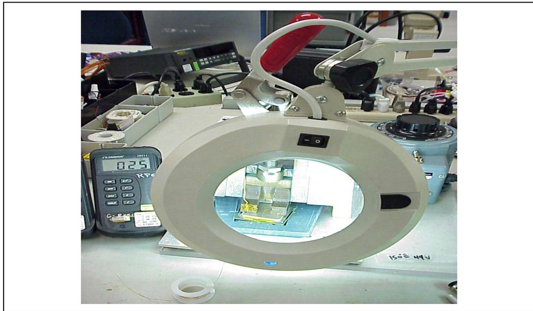
**Figure 51. Moving Solder back onto Thermocouple Bead**
