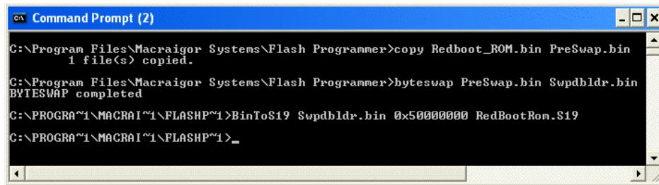
7. Now that the connection is verified, the image is byte-swapped and converted to the appropriate (.s19) format, the programmer is configured with a correct configuration file and updated for this particular flashing to be BIG ENDIAN, and the next step is to program the flash. You can choose the Erase option to erase prior to programming as shown below. Click the Program button. Wait for the progress bar to go through Erase followed by Program / Verify operation (not shown here).
