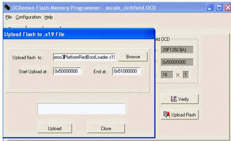
3. The flash gets erased. The following screens show stages of completion of the Programming/Verifying operation.
