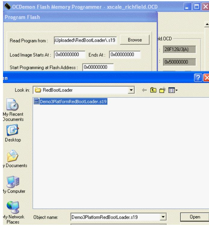
3. Provide the start and end address of the flash device; refer to the flash tab of the flash programmer menu to determine the end address from the last sector address and the size of the sector.
