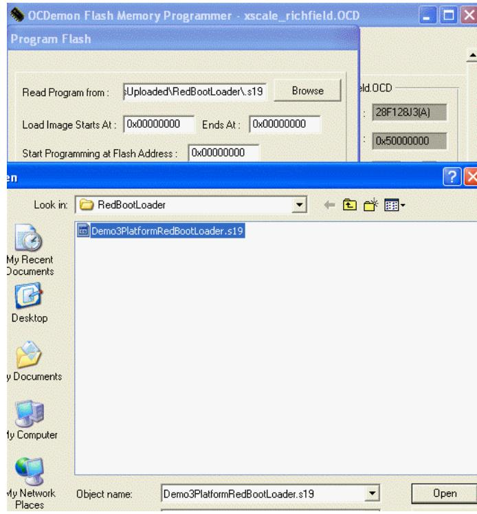
2. Note that the start and end address automatically loaded from the .s19 file.
