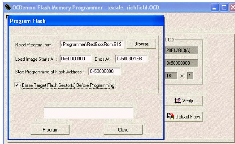
8. Wait for the progress bar to finish the Erase. The following screens show stages of completion of the Programming/Verifying operation.
