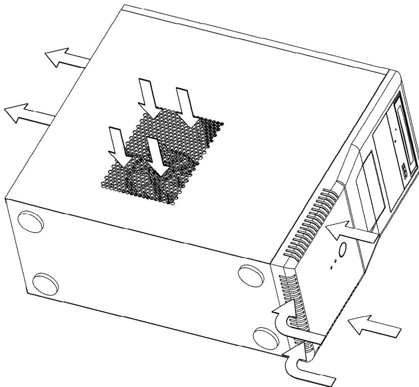
**Figure 2. Thermally Advantaged Chassis Typical Airflow Pattern**
