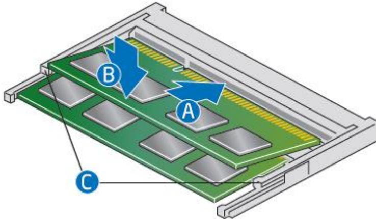
3. Align the small notch at the bottom edge of the SO-DIMM with the key in the socket.
