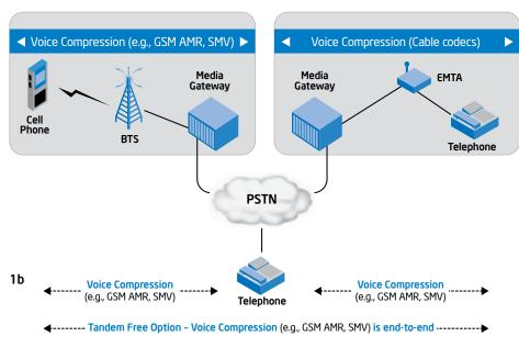
**Figure 1: Tandem Free Operation.** A cellular-to-EMTA call undergoes a minimum of two transitions (a) when voice encoded at the EMTA using a cable voice codec is converted to a cellular codec like GSM. By employing tandem free operation (b) where a Puma-4 based EMTA uses the native codec of the device it is connected with, the EMTA avoids multiple compression and decompression stages, and maintains maximum call quality.
