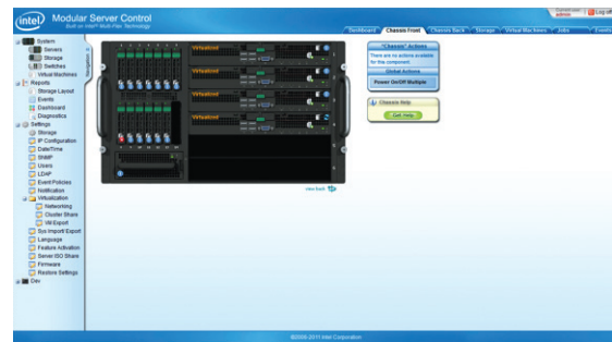
The Virtual Presence Modular Server Control allows you to see the components you physically have loaded in your system-even if they are powered down
