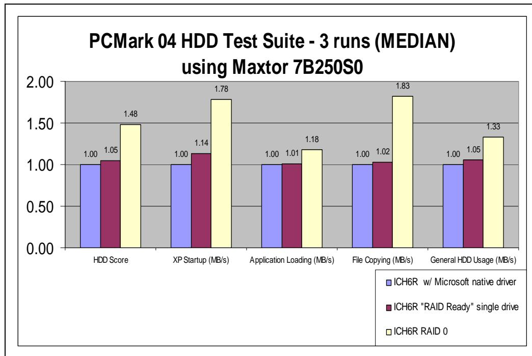
The focus on the results for this storage comparison will be on the HDD Test Suite for the PCMark 04 benchmark. The HDD Test Suite has four, separate sub-tests within the suite along with a calculated overall score (HDD Score).
