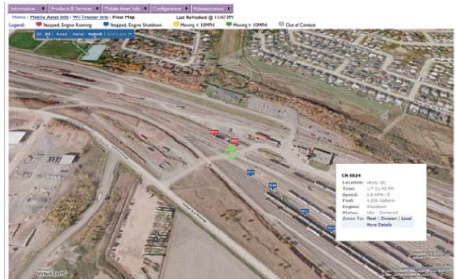
This railway monitoring system by Wi-Tronix allows an operator to locate any car via GPS tracking and see the car's contents, its destination, routing and also monitor the critical mechanical systems to anticipate maintenance requirements.
