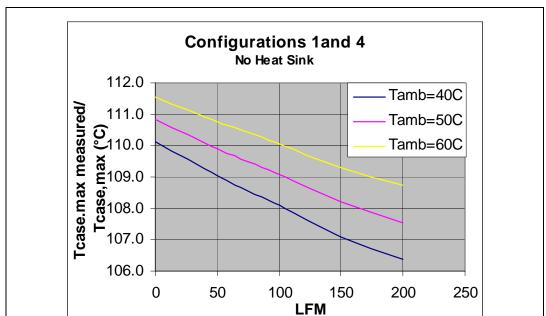
Figure 5. Heatsink Determination Chart (Configuration 1 and 4)
