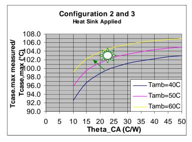
Compare the final measurement data point to Intel's  $T_{C_{max}}$  specification line (as a function of your measured ambient temperature = 40 °C) as indicated by the dark blue line ("Tamb=40C").
