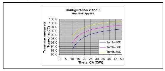
Figure 8. Heatsink Adequacy Determination Chart (Configurations 2 and 3)
