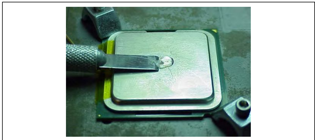
Figure 58. Removing Excess Adhesive from IHS
