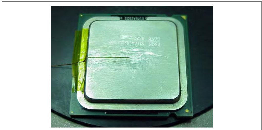
Figure 54. Thermocouple placed into groove
