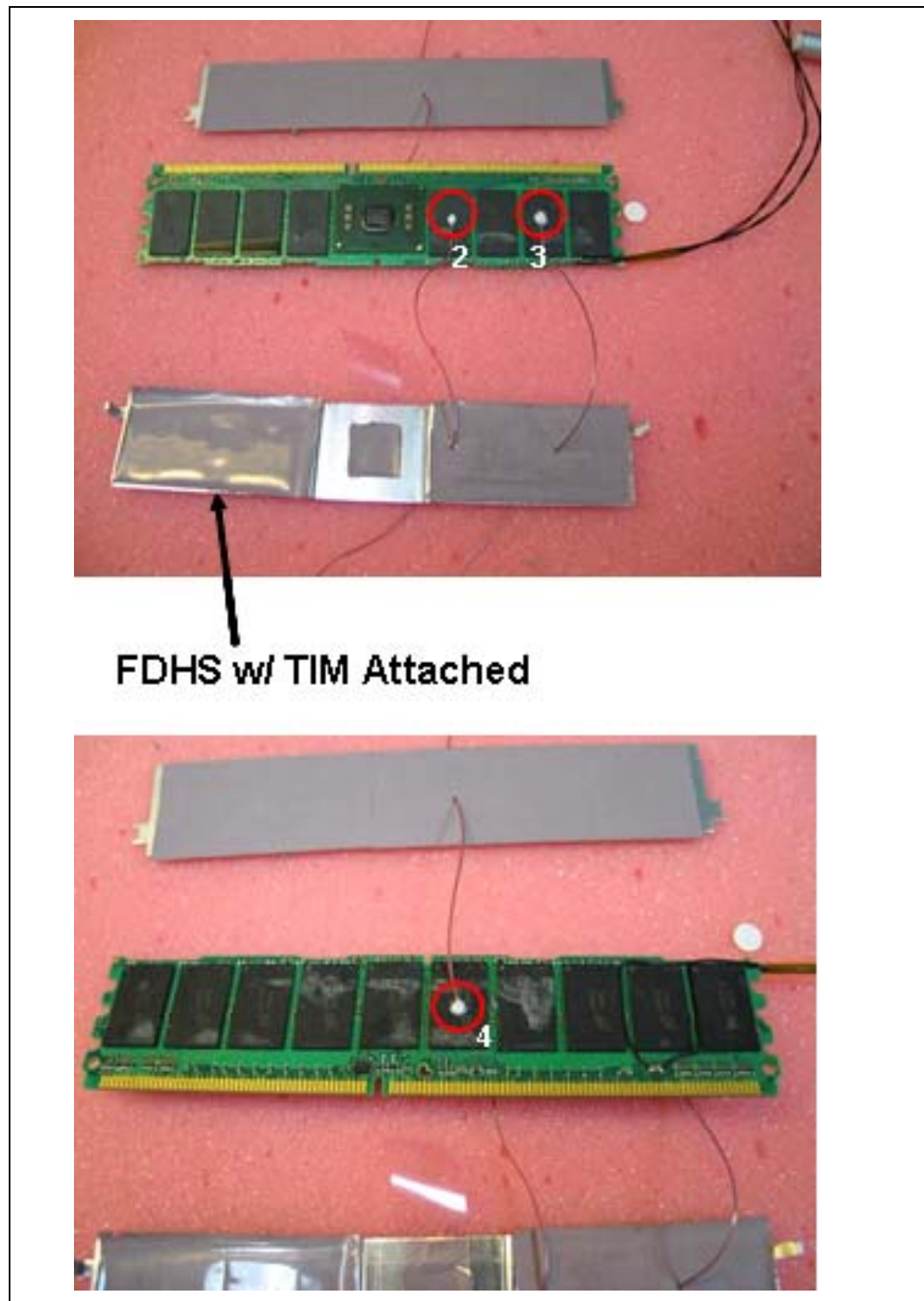
Figure 5-2. FDHS FB-DIMM with AMB/DRAM Thermocouples Attached (Pre-Assembly)
