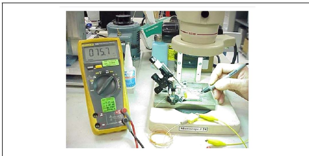
Figure 5-8. Measuring Resistance between Thermocouple and IHS
