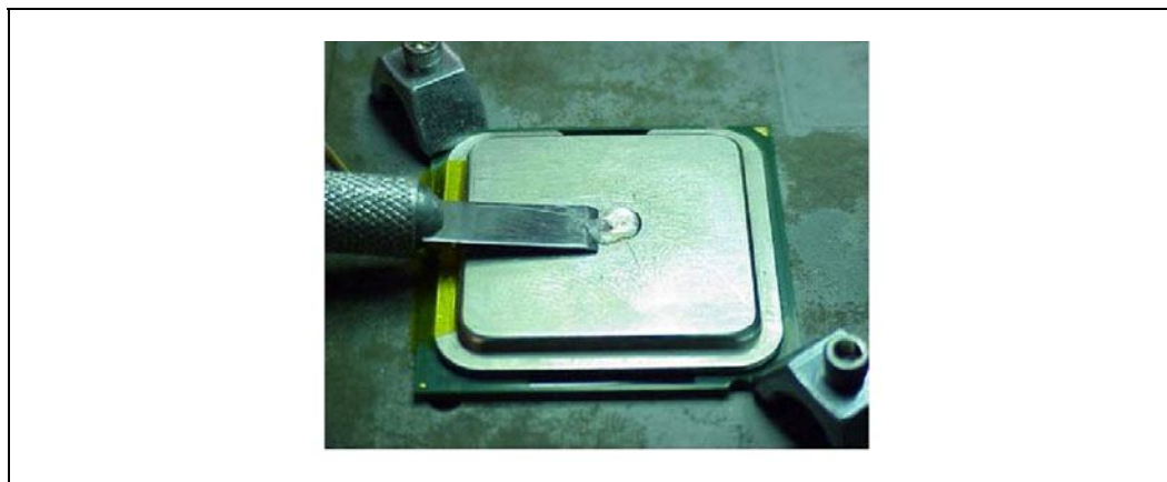
Figure 5-11. Removing Excess Adhesive from the IHS
