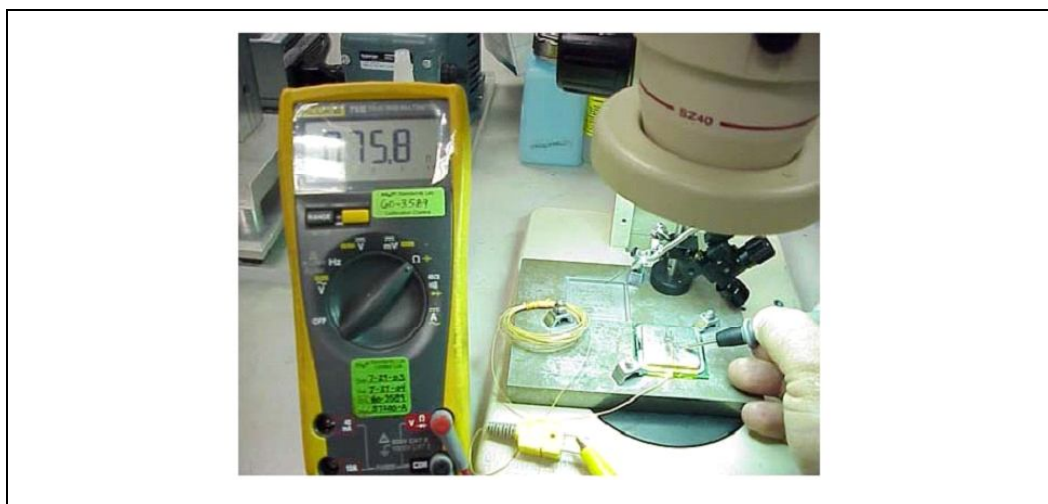
Figure 5-9. Applying in the Adhesive on the Thermocouple Bead
