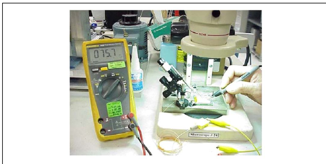
Figure 13. Measuring Resistance between Thermocouple and IHS
