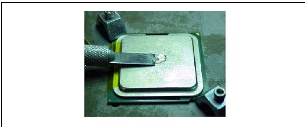
Figure 16. Removing Excess Adhesive from IHS
