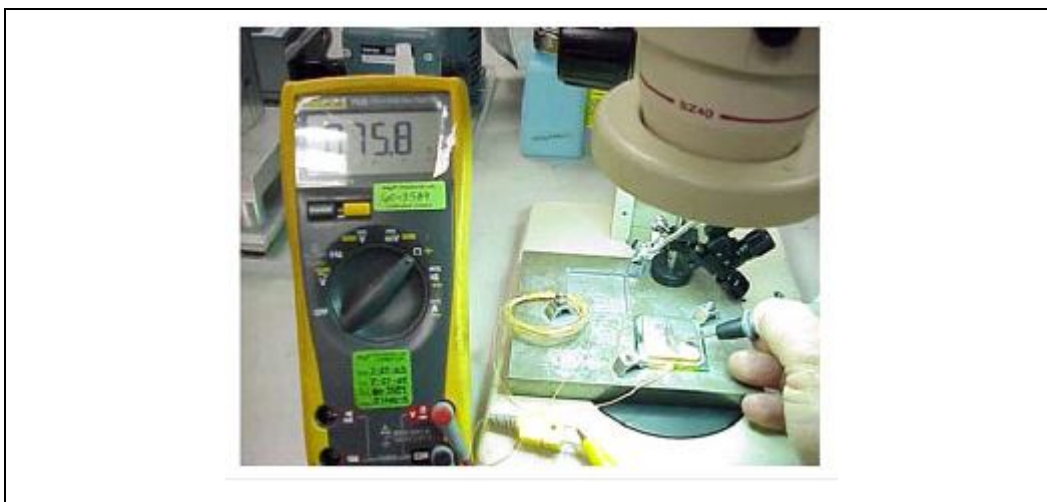
Figure 14. Applying Adhesive on Thermocouple Bead
