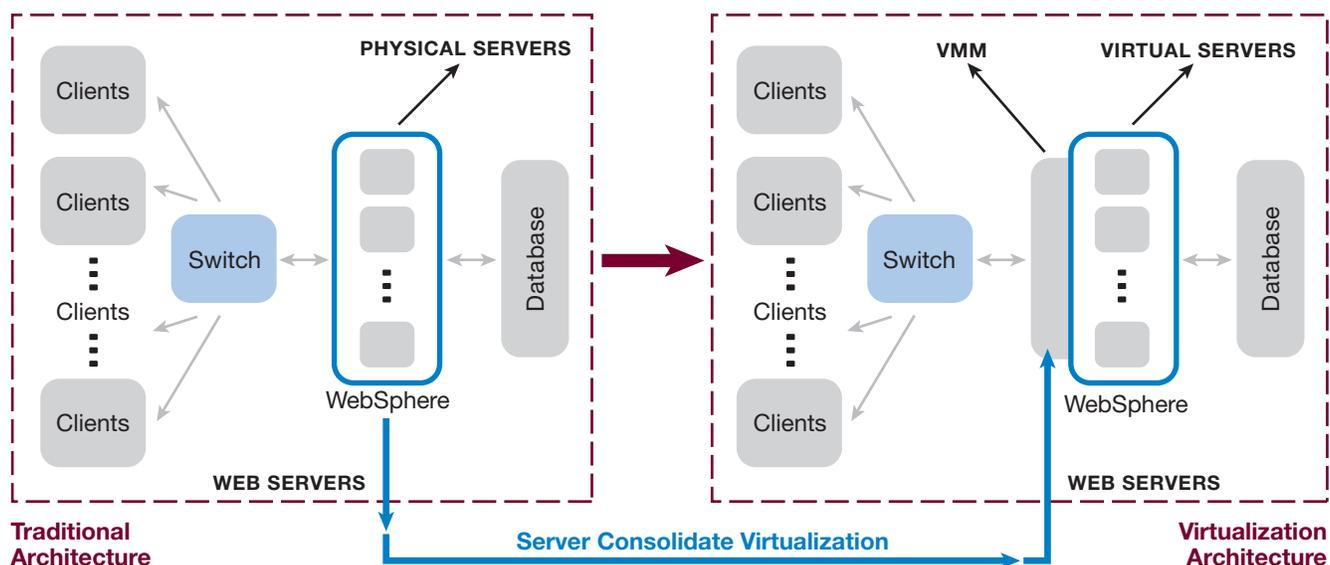
Figure 1. Neusoft Telecom BSS virtualization reference architecture.
