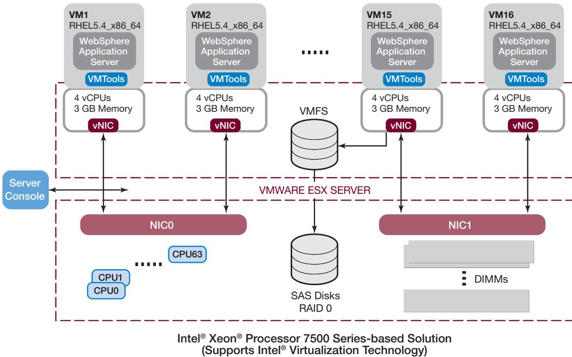
**Figure 2.** Neusoft Telecom BSS virtualization solution on Intel® Xeon® processor 7500 series-based servers.
