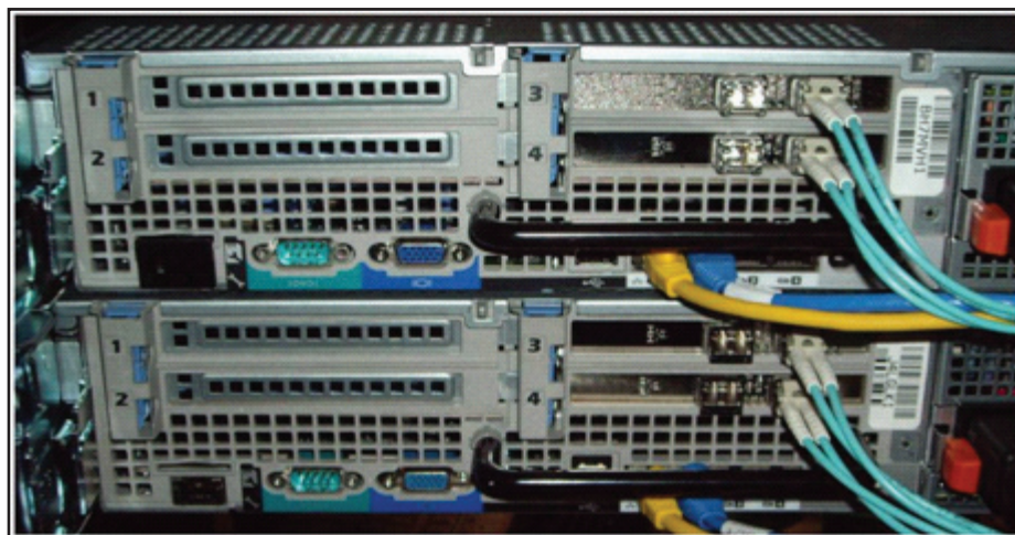
Figure 2. Simplified Server Connectivity with 10 GbE
