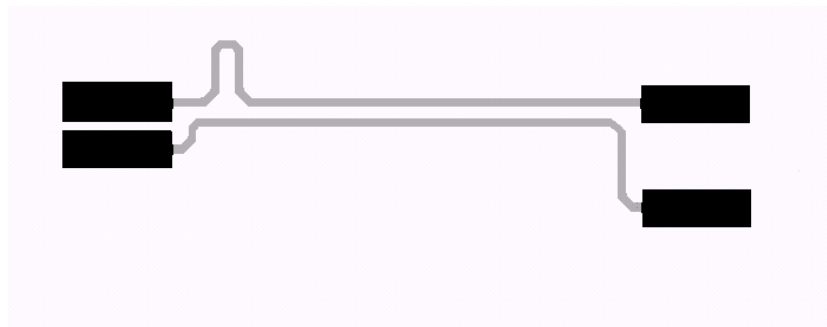
Figure 3. Poorly Routed MDI Trace Pair (Top Trace Method to Match Lengths Creates a Section That is not 100 \Omega Differential as Required)
