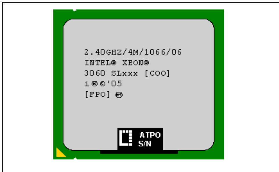
Figure 2. Processor Top-Side Markings Example for the Dual-Core Intel® Xeon® Processor 3000 Series with 4MB L2 Cache with 1066 MHz FSB
